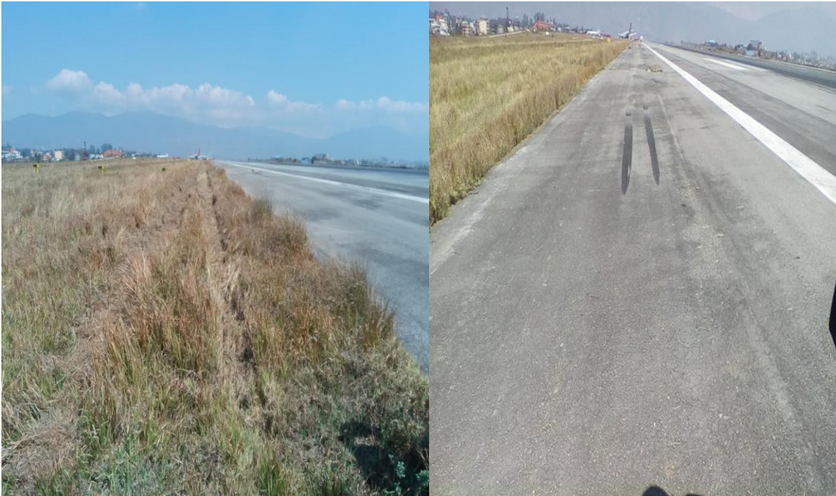
Initial touchdown points of Left and Nose landing Gears
