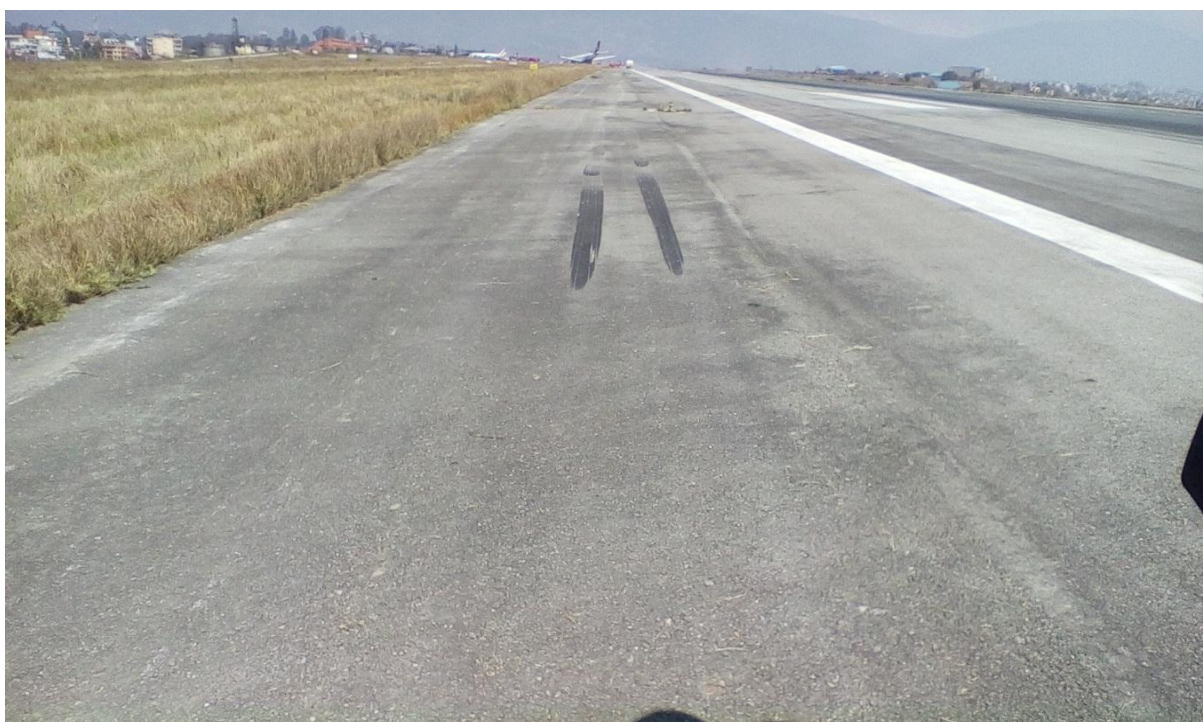
Initial touchdown point of Nose landing gear.
