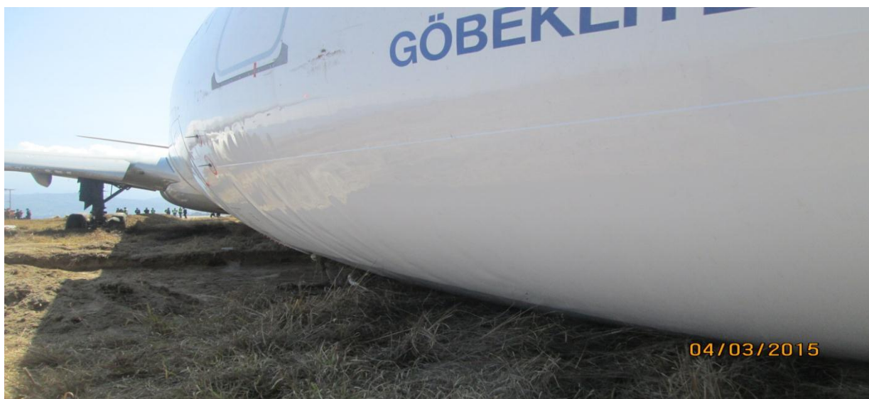
Wrinkles in the Body of the Aircraft
