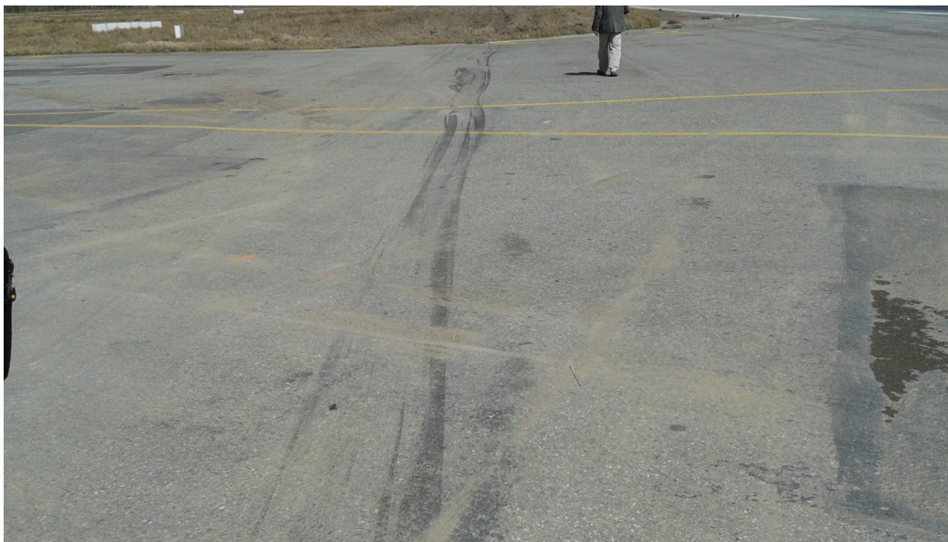
Right Landing gear Marking on the Runway just before entering into the grass area
