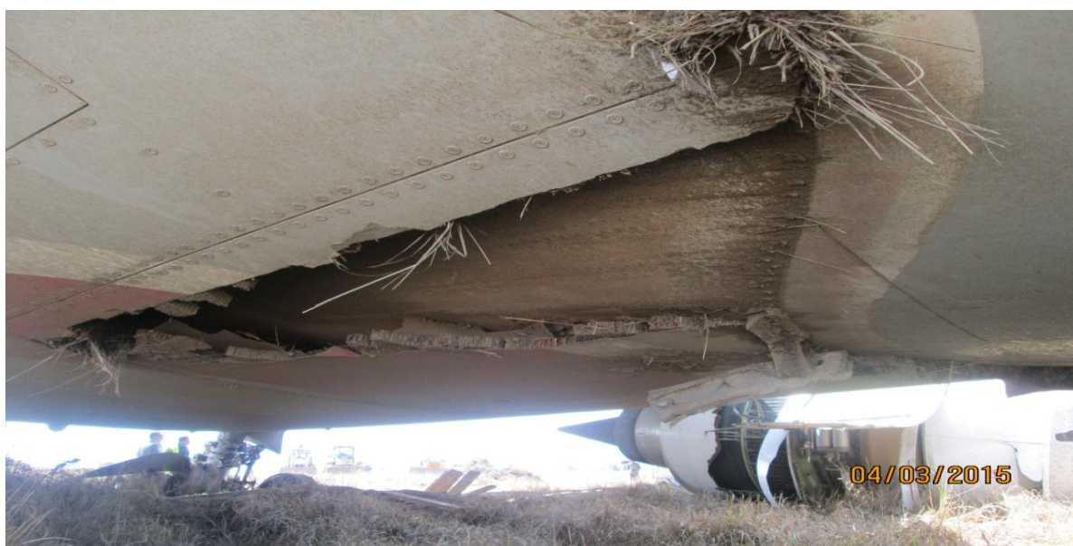
Belly of the aircraft--Fairing
